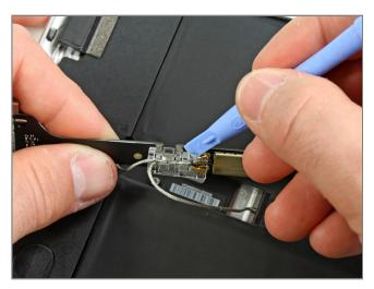
Carefully remove the plastic cover over the WiFi/Bluetooth board and dock connector cable using an iPod opening tool.
